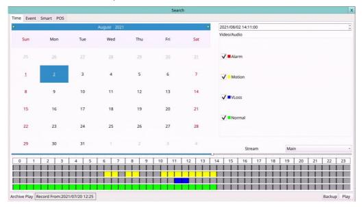
The Status field will show the 'Recorded from' time, it's based on the Video/Audio before searching. Above the status, fields are the 24H time slider and alarm/motion/video loss/normal recording status (from top to bottom).
