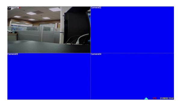
The split-window screen, as shown above, is the main screen after system startup. There are several types of split-window screens, including 1-Window, 4-Window, 7-Window, and 9-Window. The system will remember the last one before the normal shutdown (as described in <u>Section 5.7</u>) of the system. In addition to the split windows, the system time and the system states are displayed in the lower-right corner. The screen messages in the lower-left corner, shown while a certain event occurs.
