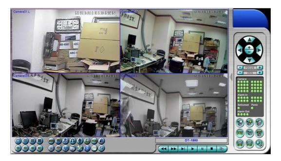
The video images can be displayed in several types of split-window screens, including 1/4/9/16-Window for single DVR and 25/36/49/64 for multiple DVRs. And the focus window is surrounded by a frame border. In addition to the video windows, there are different icons on the lower corner and the right corner of the screen for status display and control. (The ".L" following the camera title stands for Live display, ".P" for Playback, and the camera title with white background has detected motion.)
