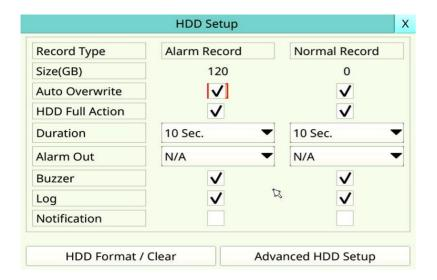
In surveillance applications, alarm video/audio is much more important than normal video/audio. So, this digital video/audio recorder is designed to allow the user to divide each HDD into an alarm partition and a normal partition. And, alarm video/audio will be recorded in the alarm partition, normal video/audio in the normal partition.
