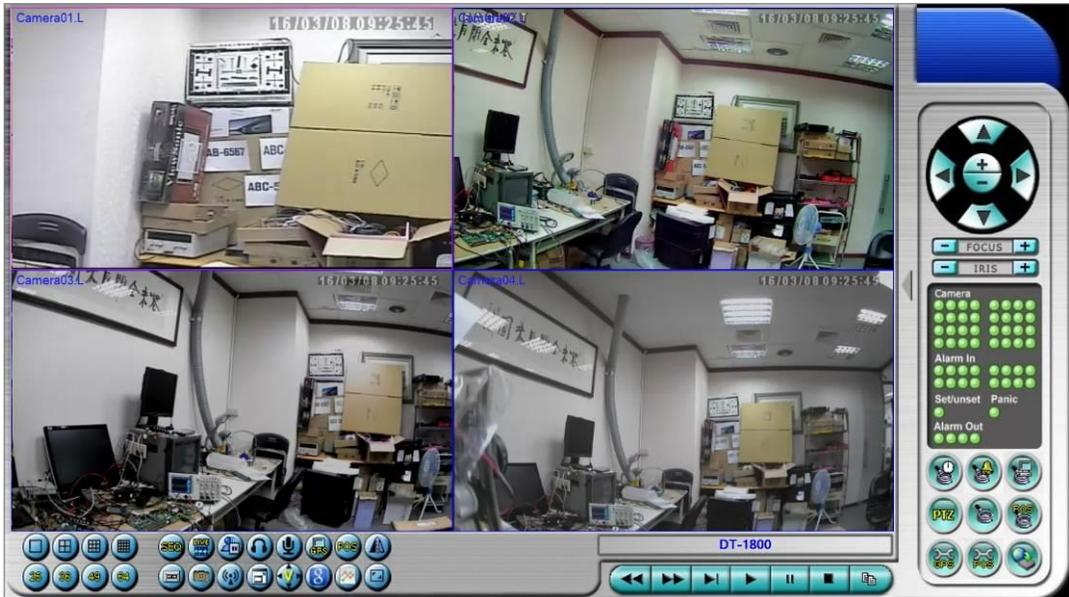
The video images can be displayed in several types of split-window screens, including 1/4/9/16/25/36/49/64 for DVRs. And the focus window is surrounded by a frame border. In addition to the video windows, there are different icons on the lower corner and the right corner of the screen for status display and control. (The ".L" following the camera title stands for Live display, ".P" for Playback, and the camera title with white background has detected motion.)
