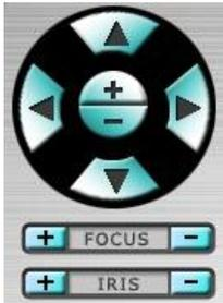
**PTZ control panel.** If the camera in the focus window is a PTZ camera, these buttons in the PTZ control panel can be used for PTZ control. The operations include Tilt Up/Down, Pan Left/Right, Zoom In/Out, Focus Near, Focus Far, Iris – (darker), Iris + (brighter).
