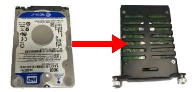
2. Plug in the HDD tray to MDVR then lock HDD gateway.
