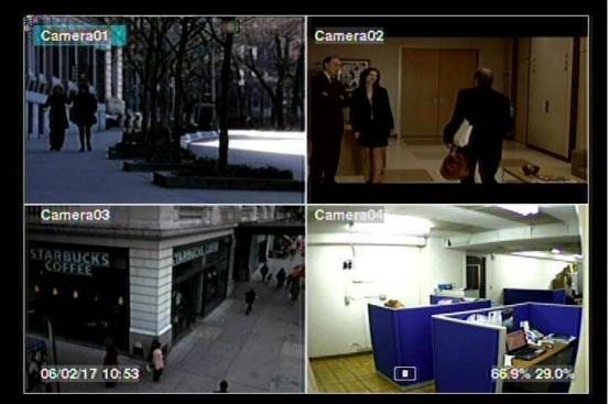
The split-window screen, as shown above, is the main screen after system startup. There are different types of split-window screens. The system will remember the last one before normal shutdown (as described in <u>Section 5.7</u>) of the system. In addition to the split windows, the system time is displayed on the lower-left corner, the system states on the lower-right corner, and the rolling screen messages, if shown while certain event occurs, on the lower corner.
