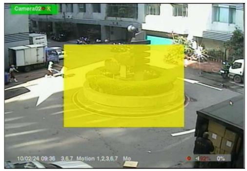
The system supports X2/X4 Digital Zoom function. To use this function, press **X2** button (Mouse: ) in full screen display to enter Digital Zoom mode. There will be a zoom window shown in the video window as shown. The zoom window (a) will always be shown at zoom factor X1, (b) can be shown or hidden at zoom factor X2, and (c) will never be shown at zoom factor X4. The operations in Digital Zoom mode are as below:
